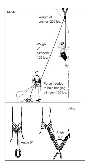
14-04a—The 100 pounds of force needed to hold the climber consists of about 67 pounds of pulling force by the belayer and about 33 pounds of force in friction at the anchor biner.
