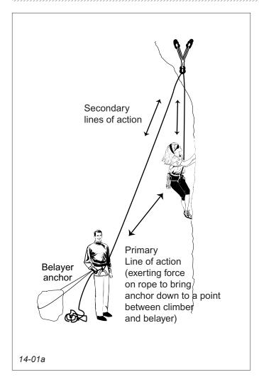
14-01a—In a slingshot anchor, the rope-bearing biners (master point) attempt to move to a position directly between the climber and the belayer.
