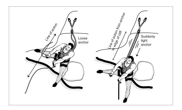
14-01d—In a seated top anchor, it is best to position your belay stance right at the edge, often with legs dangling over. Doing so puts you directly in the line of action.
